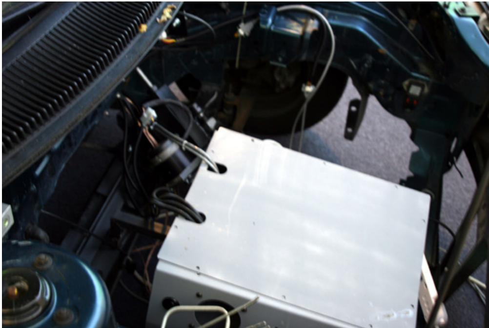
Figure 2. Junction box that distributes computerized signals to steering wheel, accelerator, brake and retrieves turn-signal indications.
