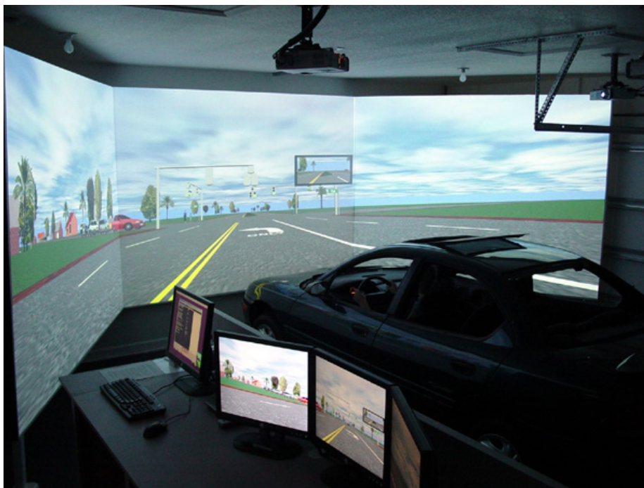
Figure 3. The Workstation overlooks the driver, vehicle and projected scenes.
