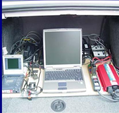
Sensors and cameras connected to a data acquisition system
