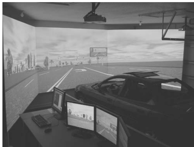
Figure 2 The workstation, vehicle, and projected scenes.
