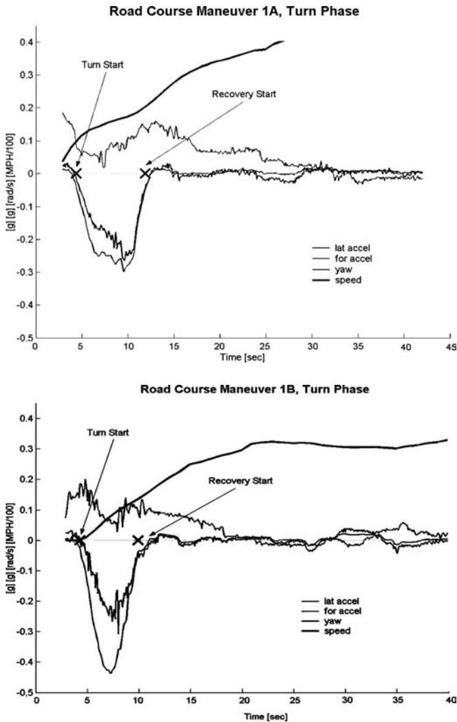
**Figure 2a and b** Graphs plotting the kinematics data for maneuver 1A (improved intersection) and maneuver 1B (unimproved intersection), indicating smaller yaw and lateral acceleration, but greater speed, as expected, for maneuver 1A (improved intersection).
