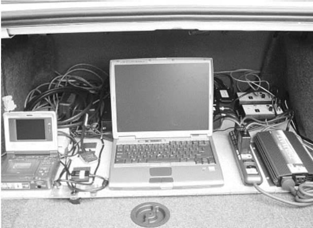
**Figure 1** Setup and recording devices in the trunk of the instrumented vehicle.
