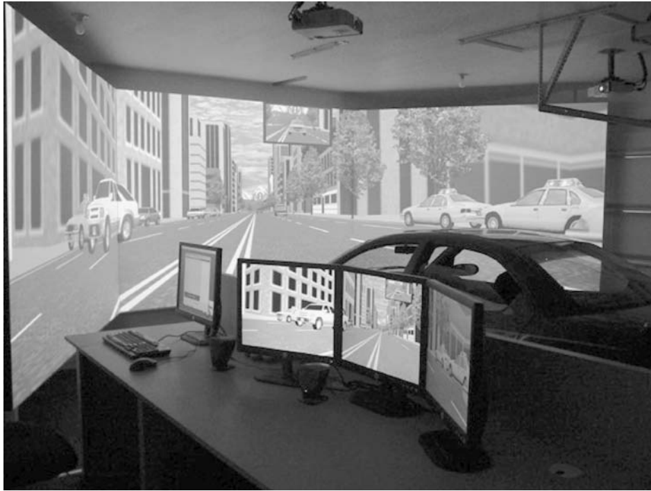
Figure 2. The workstation overlooks the driver, vehicle, and projected scenes in the driving simulator.
